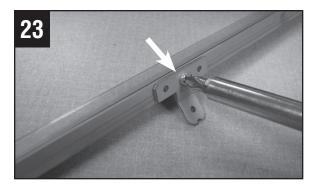
Attach the spring tension bracket on the new cleaning blade bracket. Apply lubricant to the edge of the new cleaning blade.
