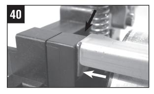
Reposition the small metal side bracket. Secure bracket with the 2 screws removed in step 5 and 6.
