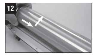
Slide the used OPC drum towards the front and lift out to remove.
