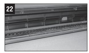
Vacuum and clean the cleaning unit and drum unit frame.
