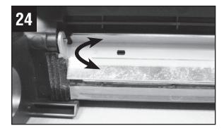
Position and secure the new cleaning blade into the drum unit frame. Confirm proper pivot movement of the cleaning blade.
