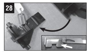
Remove the comb electrode by removing the spring tension pivot bracket from the corona end block.
