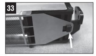
Release the spring tension and attach the screen grid mesh to the pivot bracket. Reposition the corona cleaner back to home position.
