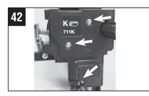
Install the front cover and secure with the 3 screws removed in step 3.
