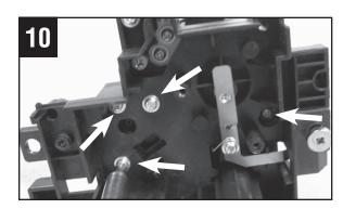
Remove 4 screws from inner front frame.
