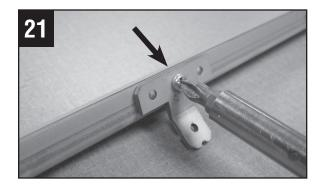
Remove the spring tension bracket from the used cleaning blade.
