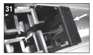
Remove the paper guide used in step 29 from the comb electrode pinch cleaner. Install the charge screen grid mesh cleaner.
