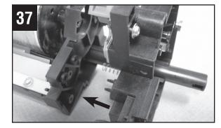
Slide inner front frame on drum unit while aligning the OPC drum pin and charge corona unit positioning pins.
