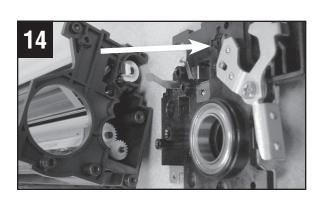
Remove the rear frame plate.
