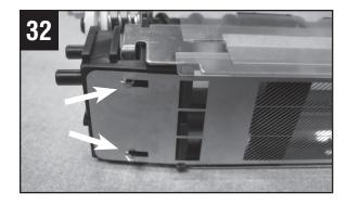
Attach the new charge screen grid mesh on the corona end block.
