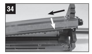
Install the charge corona unit into the drum unit frame.
