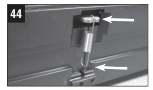
Install the drum cleaning blade tension spring.
