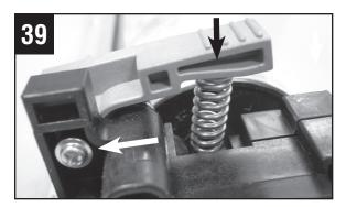
Position latch spring. Compress latch and tighten stop screw.
