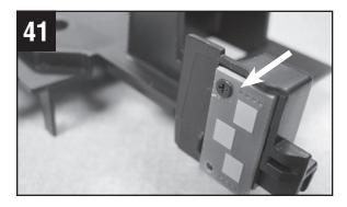
Install the new reset chip on the front cover.
