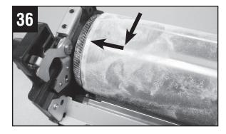
Carefully position the new OPC drum into the drum unit frame.
