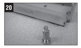
Remove the used drum cleaning blade (1 shoulder screw shown).
