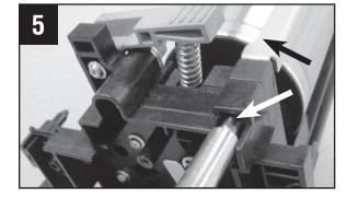
Remove the front screw securing the small metal side bracket.
