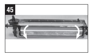
Manually rotate the OPC drum in the direction shown to clean lubricating powder from drum surface. Rotate OPC near the ends, do not touch the OPC coating.
