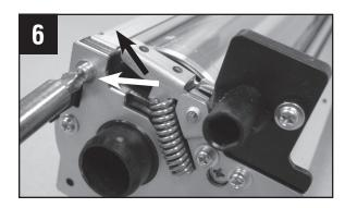
Remove the rear screw securing the small metal side bracket.
