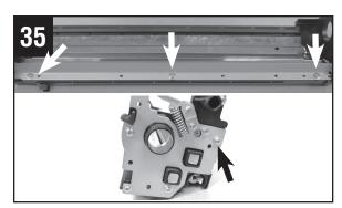
Reposition and secure the metal side bracket.
