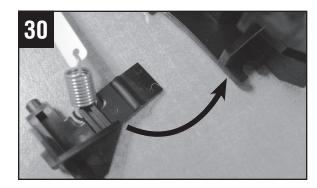
Connect the tension spring to the new comb electrode and reposition the pivot bracket in the corona end block.
