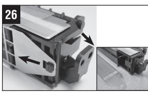
Reposition the corona cleaner away from the corona end block. Detach the charge screen grid mesh cleaner.
