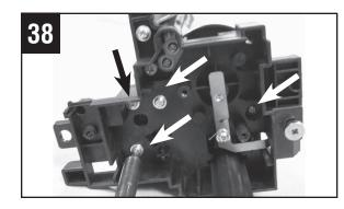
Secure inner front frame to drum unit frame using 4 screws.
