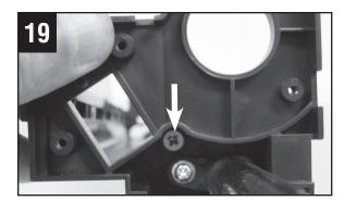
Remove the front drum cleaning blade shoulder screw.
