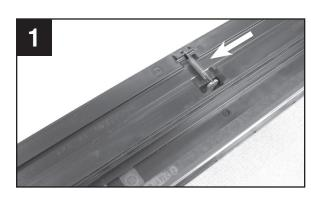
Remove the drum cleaning blade tension spring.
