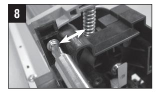
Loosen the screw to release the latch spring tension.
