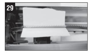
Fold a small piece of paper and position in the comb electrode pinch cleaner. The paper will aid in installing the new comb electrode. Connect metal bracket to new comb electrode and position in end block.
