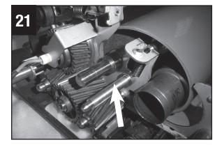
Move the foam pressure roller toward the drive side so that the larger diameter is resting on the frame.
