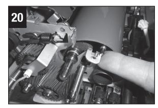
Lift the ends of the tensioner roller and place in the bushings.
