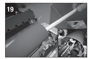
Slide the tensioner roller into the belt so that it is resting on top of the heat roller.
