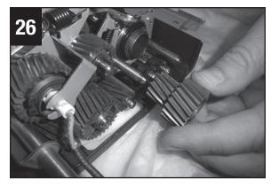
Confirm proper installation by comparing the amount of tension on each tensioner spring. They should be in the same relative position on each end.
