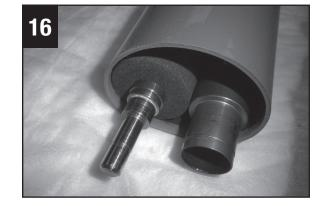
Align large diameters of rollers inside of guide ribs.
