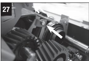
Reassemble the rest of the fuser by reversing steps 1-9. When replacing the top frame, ensure that the thermistor is securely connected, and that the wiring is placed so that it does not become pinched when the upper cover is replaced.
